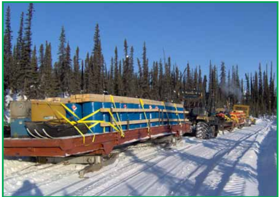
Transport equipment on winter roads using skids when the ground is frozen to avoid rutting.
