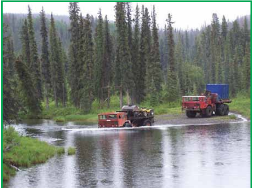
Ford streams at right angles and choose a site with gently sloping stream banks.
